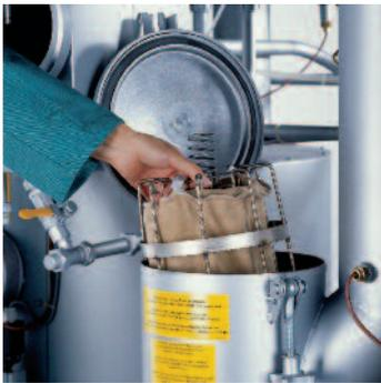
Only one maintenance opening for Lint filter and button trap: The round design eliminates edges for lint to gather
