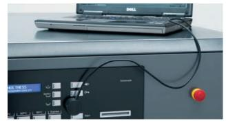
PC interface to simplify programming of wash cycles
